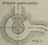
CROSS SECTION OF ADMISSION VALVE FITTED WITH OPENINGS O FOR THE PRE-ADMISSION OF STEAM.
